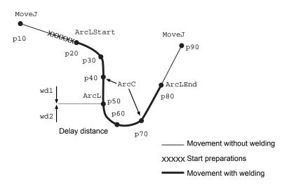
The welddata, wd1, applies until position p50 is reached, where a transition to wd2 takes place.
