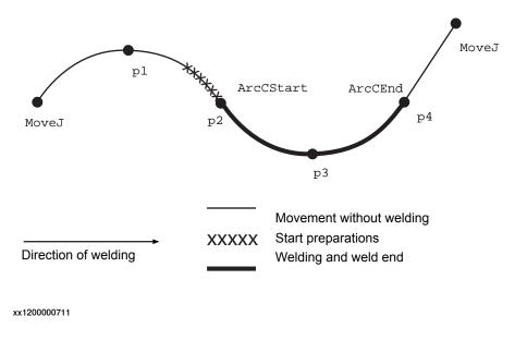
7.1.3 ArcCStart, ArcC1Start, ArcC2Start - Arc welding start with circular motion Continued
